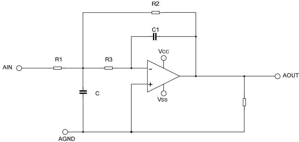
The second-order filter structure shown as above is adopted for 6-channel audio amplifier, with in-band gain of about 12dB and -3dB bandwidth of 40kHz above which is well meet audio requirements. As principle structure, in-band gain is decided by:  $G = -\frac{R_2}{R_1}$ , thus, gain can be adjusted by changing R1.
