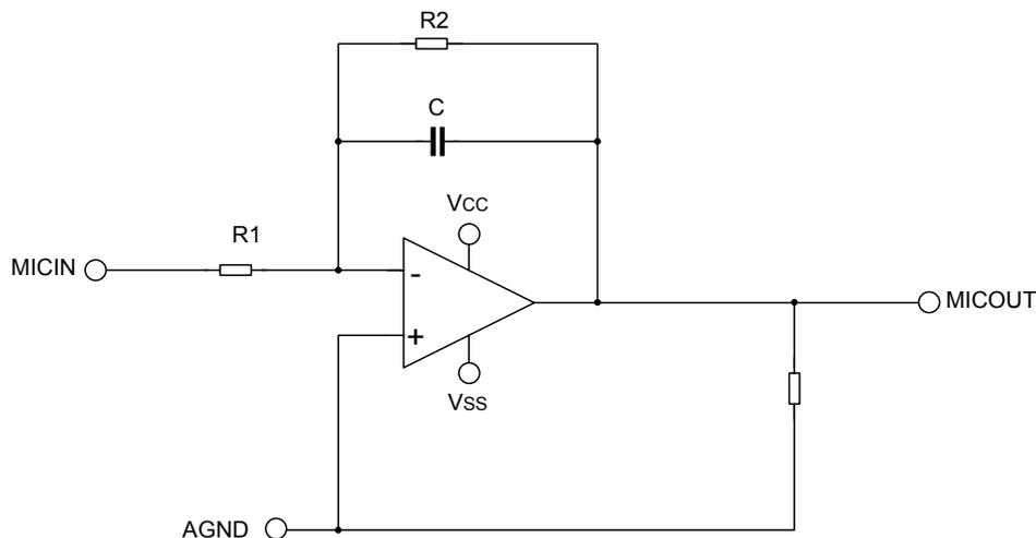
The proportional amplifier shown as above is adopted for microphone amplifier with setting gain of about 29dB, and capacitor c is used for high frequency signal filtering. As described above, the gain can be also adjusted by changing R1.
